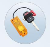
Data detection. When indicated by the cloning device, wrap the U-Snoop around the customer key and turn the key in the car ignition 2 times. U-Snoop LEDs illuminate to confirm successful sniffing.
